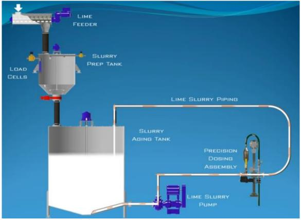
Figure 4-3: Proposed Lime Feed System
